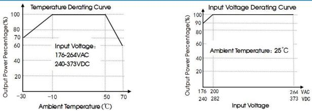
Note: ① With an AC input between 176-200VAC and a DC input between 240-282VDC, the output power must be derated as per temperature derating curves; ② This product is suitable for applications using natural air cooling; for applications in closed environment please consult factory or one of our FAE.
