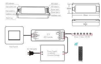
The controller could auto check and output a proper voltage according to its LED quantities.
